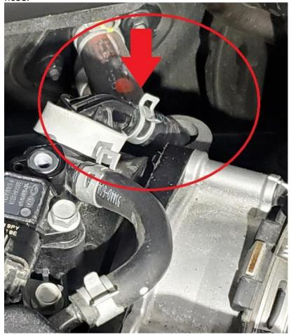
Preinstall the hose clamp on the J&L hose with the 90-degree fitting, the screw head of the clamp should be on the back side of the hose. This will help when you have to tighten it. Install this hose onto the intake manifold fitting.
