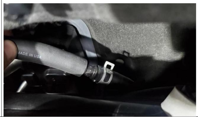
At the oil separator, connect the hose that is going to the intake manifold (the hose with the 90-degree fitting to the "C" side of the oil separator. (OSC logo) **TIP: Use light oil or grease** inside the hose end and/or on the oil separator fittings, this will allow you to easily install the hoses onto the oil separator fittings.
